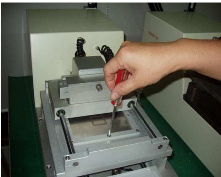
换新规格放回压片上紧螺丝
