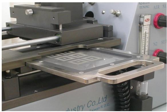
All kinds of solder ball placement tooling for BGA IC.
