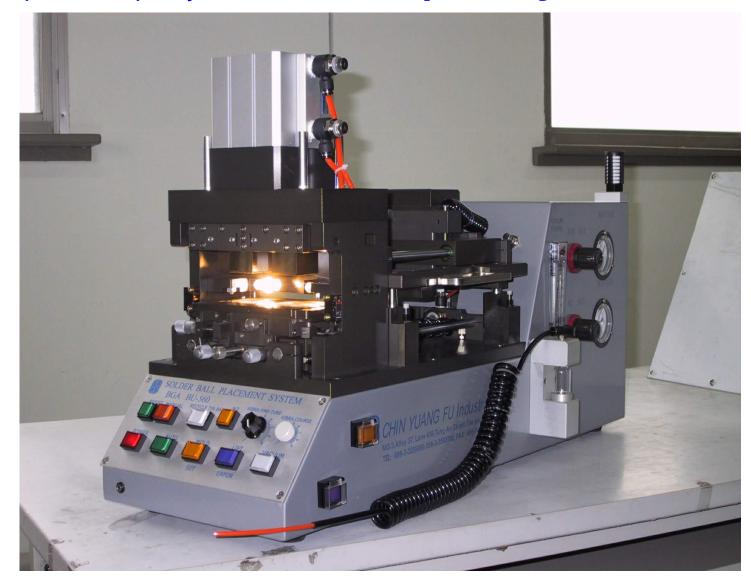
X-Y- $\theta$  Theta positioning slider with micrometers adjustment & BGA fixtures.
