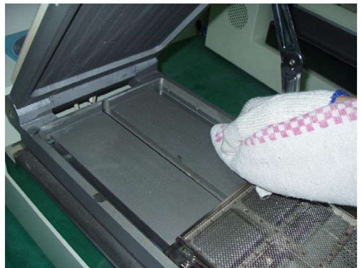
Clean the right Railing
